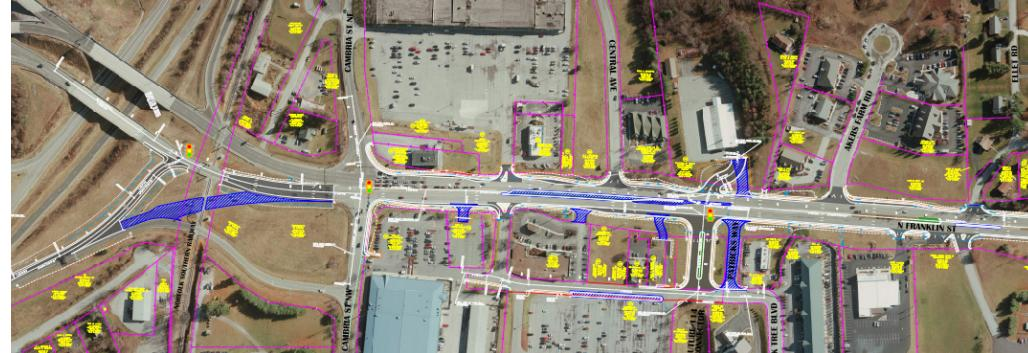
Note: Blue highlighted sections indicate areas where pavement will be removed.
