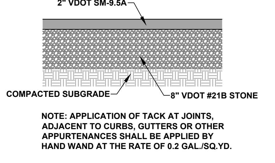
NOTE: APPLICATION OF TACK AT JOINTS, ADJACENT TO CURBS, GUTTERS OR OTHER APPURTENANCES SHALL BE APPLIED BY HAND WAND AT THE RATE OF 0.2 GAL./SQ.YD.
