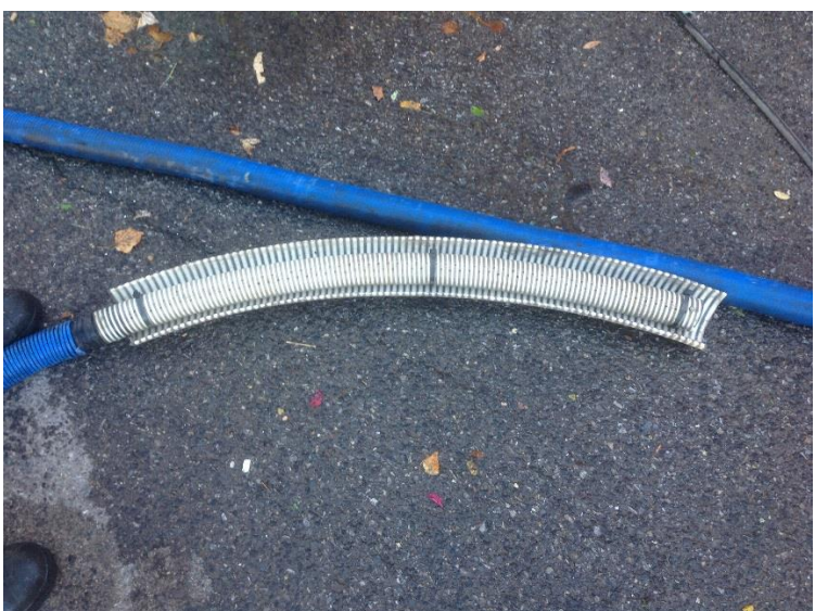
Photo 3. October 24, 2016. Suction line without filter sock.
