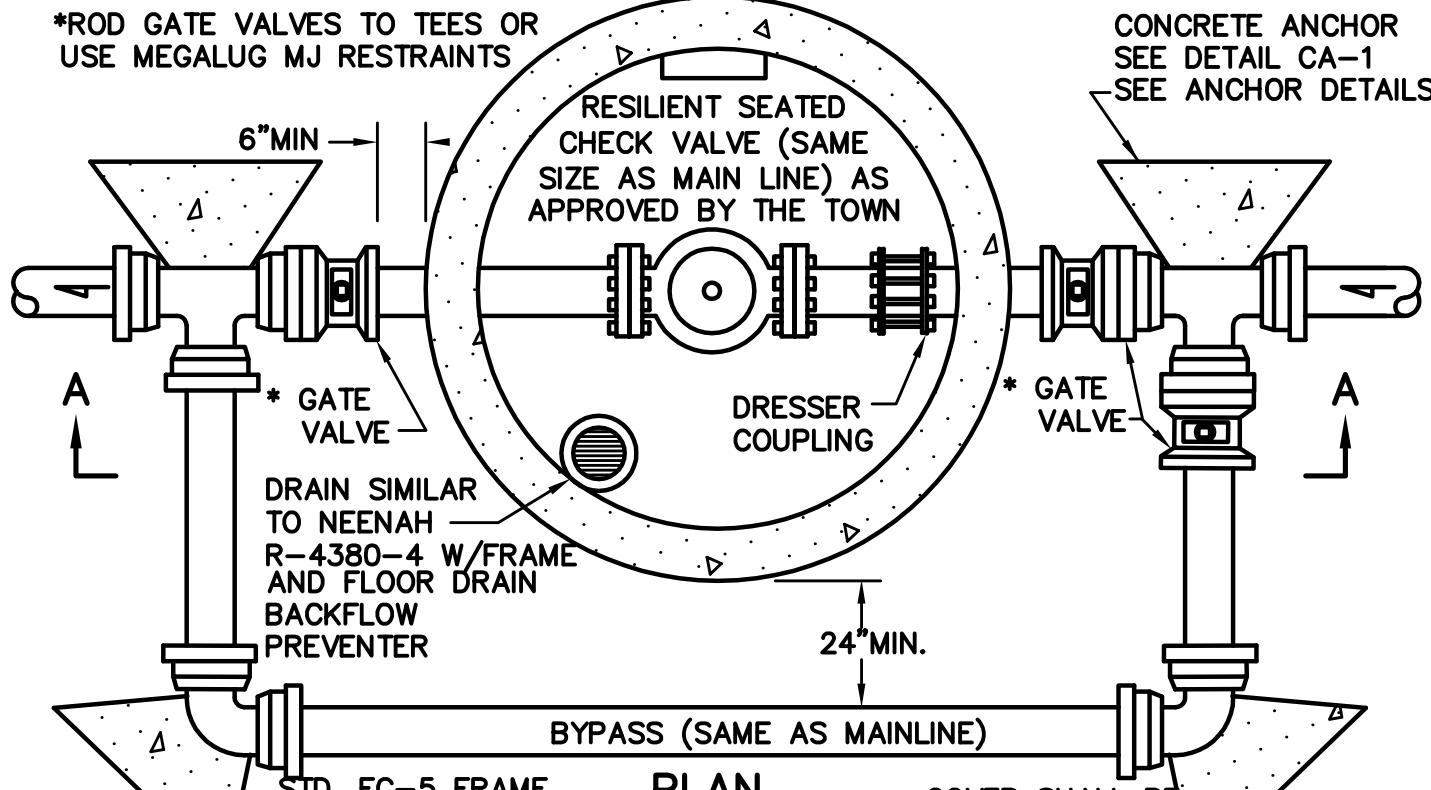
CONNECT PIPE TO SECTION WITH APPROVED WATERTIGHT SLEEVE OR GASKET
