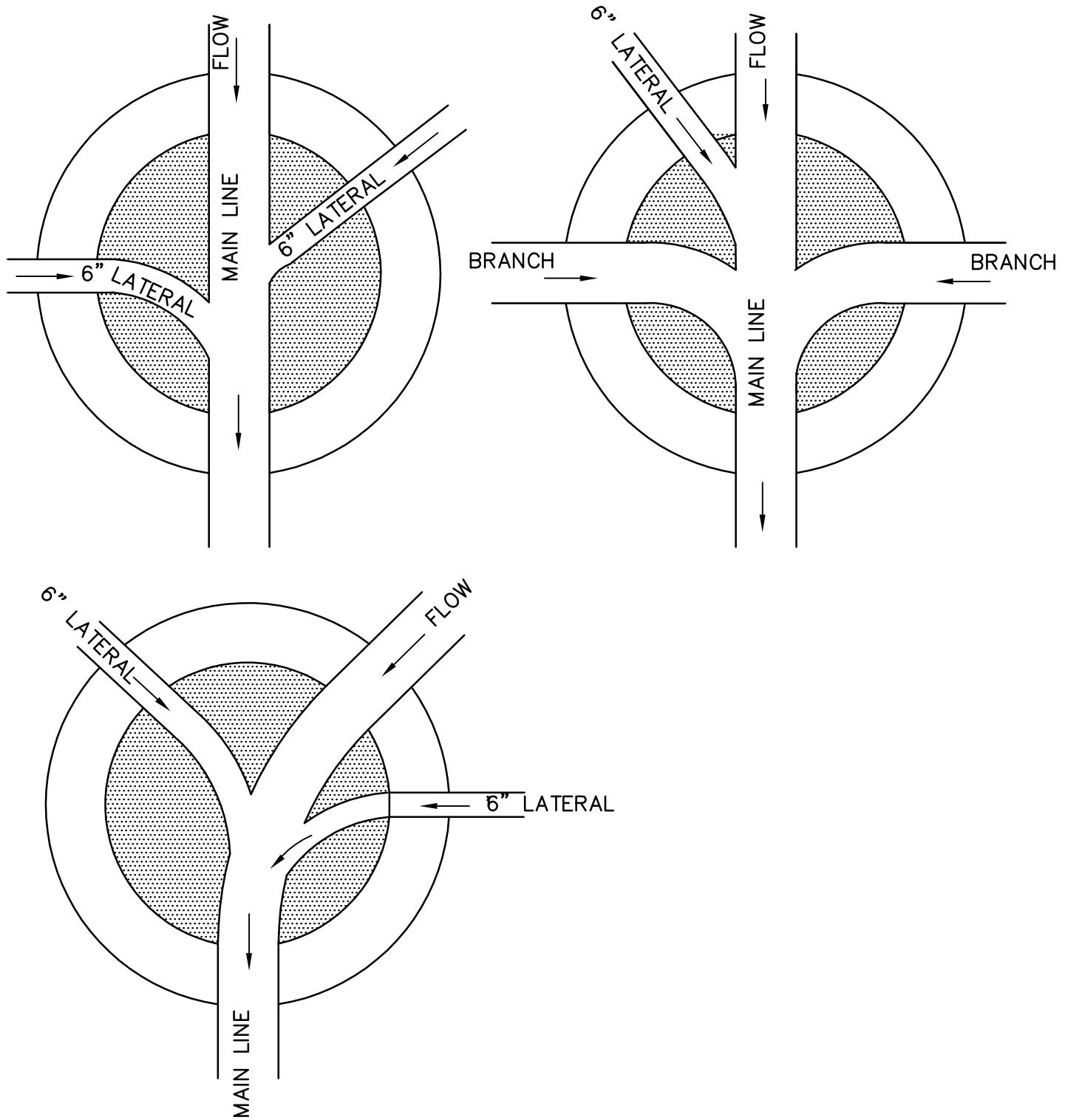
THE INVERT CHANNELS SHALL BE FORMED WITH CONCRETE AS SHOWN AND SHALL BE SMOOTH AND SEMI-CIRCULAR IN SHAPE, CONFORMING TO THE INSIDE OF THE ADJACENT SEWER SECTION. CHANGES IN THE DIRECTION OF FLOW SHALL BE MADE WITH A SMOOTH CURVE OF AS LARGE A RADIUS AS SIZE OF MANHOLE WILL PERMIT.
