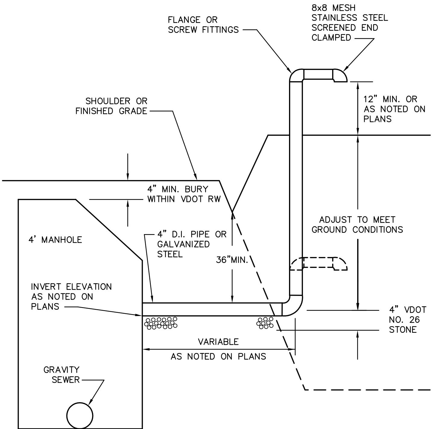
NOTE: CONNECT PIPE TO SECTION WITH APPROVED FLEXIBLE WATERTIGHT SLEEVE OR GASKET (INTERPACE OR EQUAL)
